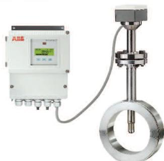
Leak detection is typically carried out at night, while the air main is pressurised but the legitimate users are off-duty. Accurate leak detection demands a meter that can measure very low flows, which is another reason to opt for thermal mass flowmeters. Thermal mass units have a turndown ratio of 150:1, compared to between 30 or 40:1 for vortex meters and just 4 or 5:1 for orifice plates.
