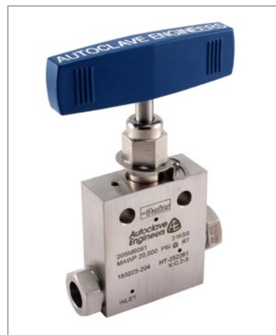
Parker Autoclave Engineers needle valve (20SM Series) ISO 19880-3 certified for hydrogen refuelling stations. Temperature range: -73°C to 316°C (-99°F to +601°F) MW Pressure: up to 700 bar (10,152 psi).
