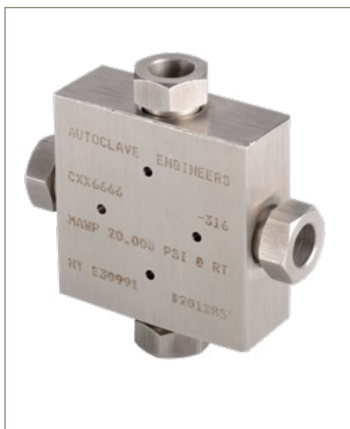
Parker Autoclave Engineers cone and thread fittings EC-79 approved for on-board hydrogen-powered vehicles. Temperature range: -40°C to +120°C (40°F to +248°F) MW Pressure: up to 700 bar (10,152 psi).
