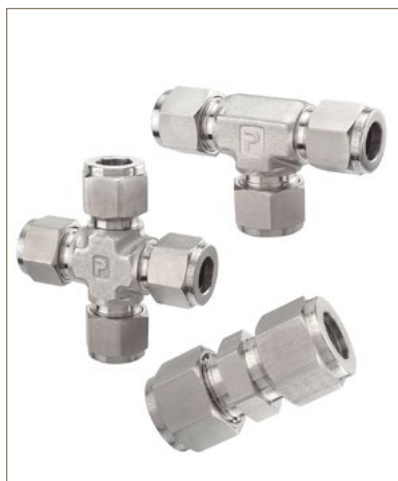
Parker two ferrule fittings (A-LOK® Series) EC-79 approved for on-board hydrogen-powered vehicles. Temperature range: -40°C to +120°C (40°F to +248°F) MW Pressure: up to 350 bar (5,076 psi).
